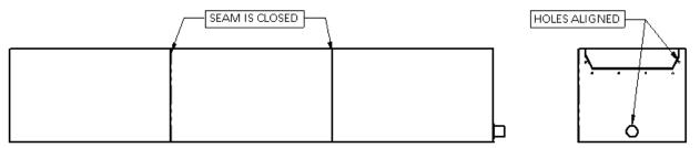
With the planter modules aligned, temporarily clamp together. Drill ½" diameter holes through both walls along the scoop out. Holes should be between 1-2 inches away from the edge of the scoop edge and spaced every 8-12 inches. The first and last holes should be as high up the wall as possible. Seal each bolt, on both sides, with SikaFlex 1A or other waterproof sealant before tightening. Remove clamps.
