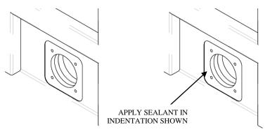
Install the flow through assembly. Threaded rods will go through both planters. Tighten (hand tight is sufficient) nuts onto threaded rods, alternating between opposing corners to ensure even pressure. Apply Sikaflex 1A to base of seal and hardware.
