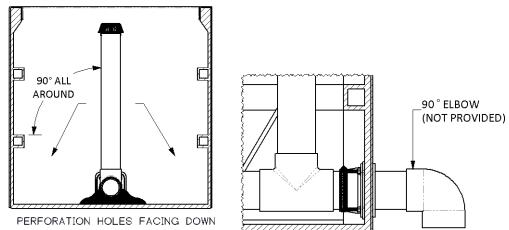
Install the discharge assembly. This can vary greatly from one project to another. Refer to your site plans to confirm discharge arrangement. Shown above is one of three typical set-ups (end elbow).
