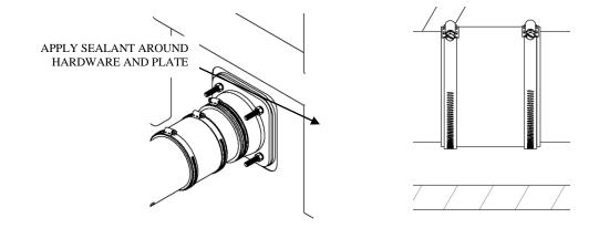
Attached glued plumbing pieces to the flow assembly using the couplings provided. Hand tighten screws on clamps to create seal. NO glue/sealant is required.
