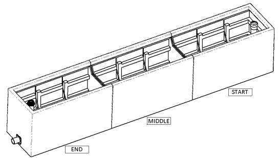
Reference layout drawings for location and quantity of planters. Place the first planter and ensure it is leveled to your specifications. It's important that the planter is fully supported and will not shift once loaded.
