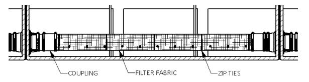
Use drainage media to support the plumbing while making sure proper slope is accounted for (refer to your site plans). Aim to have flow-through pipes centered into the hole in planter. Even spacing makes sealing around the pipe easier and more consistent.
